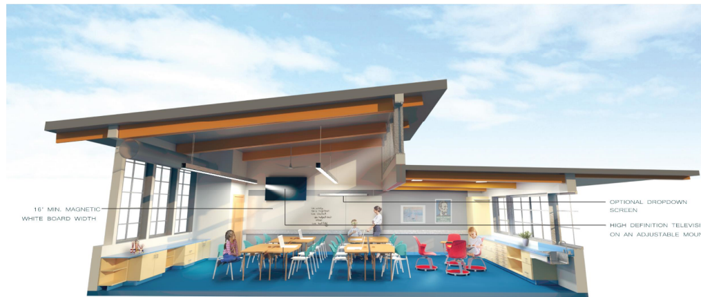
TYPICAL EXISTING CLASSROOM: CUT-AWAY SECTIONAL VIEW
